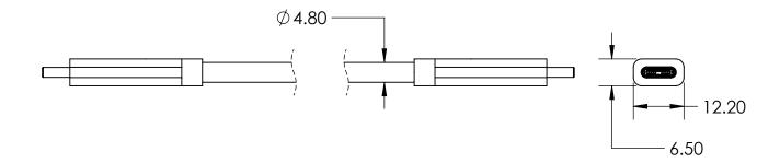
**Product:** FireNEX-uLINK USB 40G Active Repeater Cable Overmold Version, Type C Male to Type C Male, 4M Meters.
